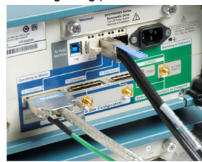
UltraSync connection on instrument with Master role
