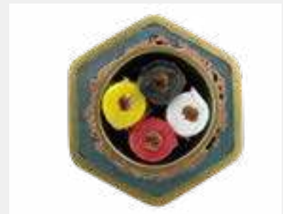
Shielded 4-wire "twisted pair" data-cable, crimped without trapezoidal indent
