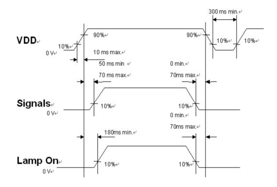
VDD power and lamp on/off sequence is as follows. Interface signals are also shown in the chart. Signals from any system shall be Hi-Z state or low level when VDD is off.
