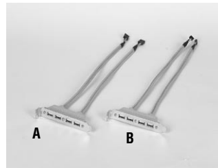
A. P/N 1700000719 Cable USB 4 ports/10P-2.54 mm * 2 30.5 cm
