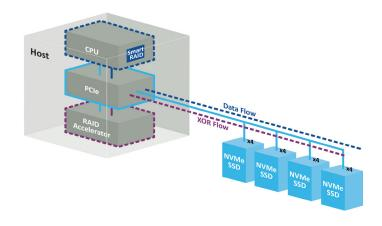
The SmartRAID 4300 maintains the enterprise-class features, functionality and hardware offload of our previous-generation in-line products, while delivering accelerated high performance that scales with the host, interconnect and CPU-attached NVMe endpoints. Management of the CPU-attached NVMe endpoints removes the dependencies that drive form factors, connector types and backplanes can create.
