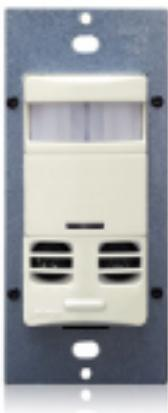
Discontinued Product. Product Line: OSSMD, Technology: Multi-Technology PIR/Ultrasonic, Switch Type: Single-Pole, Dual Relay, Fan Model, Mounting: Wall Switch, Device Type: Occupancy Sensor, Coverage (Sq.Ft.): 2400 Sq. Ft., Pattern: 180°, Color: Light Almond, Neutral Wire Connection: Required, Domestic Content: Made in USA, Warranty: 5-Year Limited
