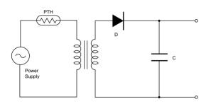
(2) Transformer Protection Circuit 2)
