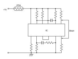
(4) Short-Circuit Test of Electrolytic Capacitor
