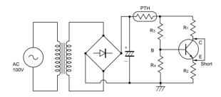
(2) Short-Circuit Test of Diode
