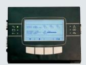
MultiPanel is a remote monitoring device that can provide a detailed UPS status overview in real time. It is compatible with all Riello UPS and can display values for UPS specific input and output supplies, and battery set measurements.
