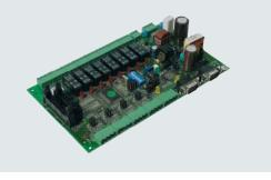
Multi I/O has configurable input and output signal contacts to allow UPS integration with control systems. It can be used to connect two devices to a single UPS serial communication port. It can also communicate using the MODBUS/JBUS protocol on RS485 lines.
