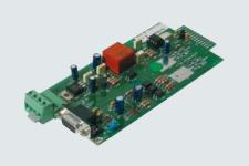
MultiCOM 372 provides a UPS with an additional RS232 serial interface port. The card has Emergency Power Off (EPO) and Remote Shut Down (RSD) inputs with terminal connections.
