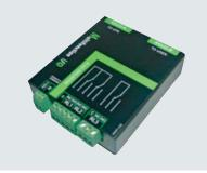
Multifunction I/O is a Dialog plus range accessory through which you can monitor battery operation, by-pass, alarm and battery discharged status reports with dry contacts (maximum current 8A/250V). The accessory also has an input which is used to set up the configurable remote on, remote off and remote on/off functions through the UPSTools software (vers. 1.3.3 or higher).
