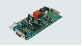
MultiCOM 362 provides a UPS with an additional RS232 serial interface or USB port. The USB port allows the UPS to communicate with Apple Macintosh computers as well as Windows and Linux operating systems.
