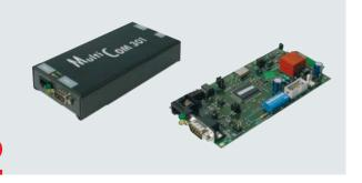
The MultiCOM 301/302 protocol converter may be used to monitor the UPS using the MODBUS/JBUS protocol on RS232 or RS485 serial lines. It can also manage a second independent RS232 serial line that can be used to connect to other devices such as the Netman 101 or a PC using PowerShield<sup>3</sup> software.
