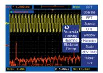
Display and measure the input signal's frequency spectrum. Select one of the 5 FFT windows: Rectangular, Hanning, Hamming, Blackman, and Flattop. Use cursors to measure the spectral component's magnitude and frequency.
