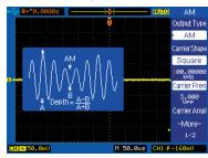
Display a graphical illustration explaining the parameters of the built-in arbitrary waveforms and modulation schemes. This is a convenient tool for students and new users.
