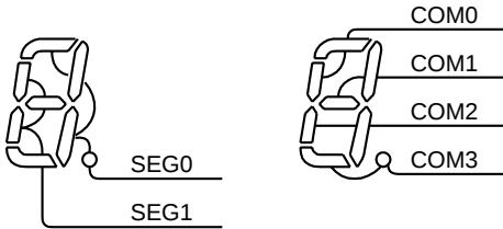
Figure 15-6 Example of COM, SEG Pin Connection (1/4 Duty)
