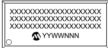
28-Lead UQFN (4x4x0.6 mm)
