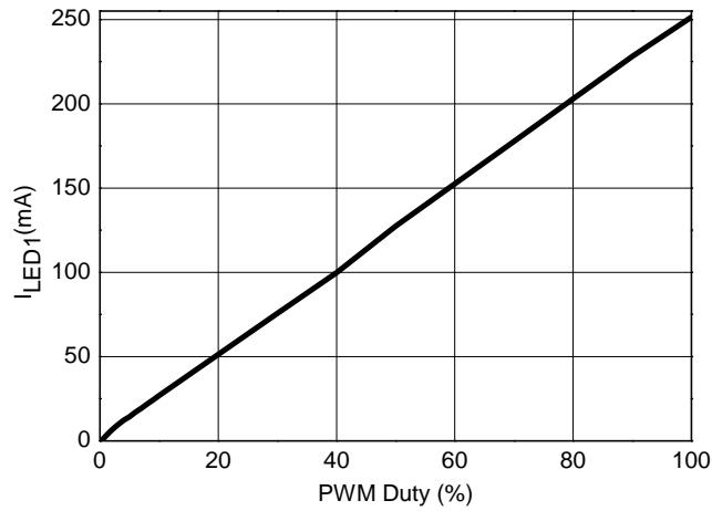
LED Current (AL1782) vs. PWM Duty (f=500Hz, 0~100%)
