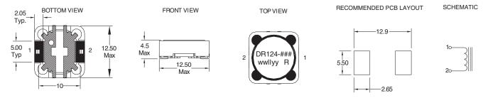
Dimensions are in millimeters.
