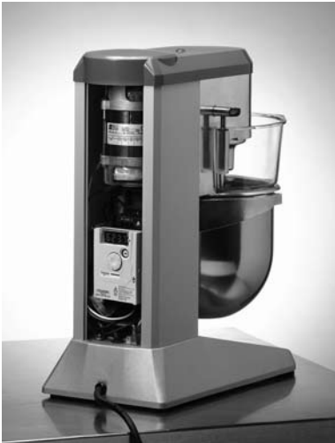
ATV12 drive controlling a mixer
