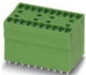
Header, Nominal current: 8 A, Rated voltage (III/2): 160 V, Number of positions: 2, Pitch: 3.81 mm, Color: green, Contact surface: Tin, Assembly: Soldering, In combination with MCV plug components, both an MCVW and an MCVR plug must be used.
