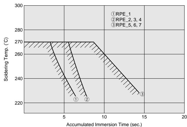
Perform soldering within tolerance range (shaded portion).
