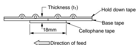
Match the separated base tapes, and connect the back side with cellophane tape.
