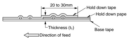
Overlap the hold down tape. Ensure that thickness (t1) does not exceed 1.05mm.
