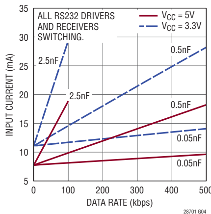
V_{CC} Supply Current vs RS232 Data Rate
