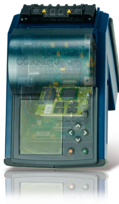
CORNING Cable Systems GmbH: glass fiber splicing unit PHYTEC contribution: development of customized hardware, application of standard modules
