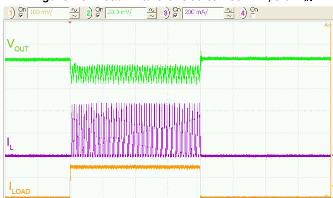
Figure 30. Load Transient 0 to 150 mA, 4.5 V_{IN}
