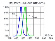
FIG.4 RELATIVE LUMINOUS INTENSITY VS. WAVELENGTH.
