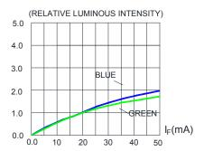
FIG.2 RELATIVE LUMINOUS INTENSITY VS. FORWARD CURRENT
