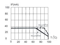
FIG.5 Blue MAXIMUM FORWARD DC CURRENT VS AMBIENT TEMPERATURE (Tjmax=110  $^{\circ}\text{C})$
