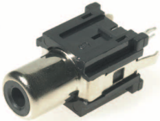
PHS-4B Snap In PCB mounting RCA Phono connector. Only available with black insert. PHS-4B (FC68375)
