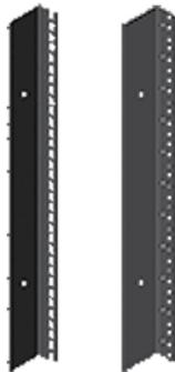
Made of 14 gauge steel with square holes or 12 gauge steel with 10-32 tapped holes. Provides 19- or 23-in. rack spacing depending on frame width. Finished with flat black RAL 9005 polyester powder paint or plated. Furnished in pairs.
