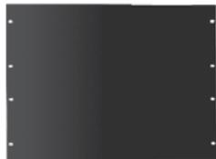
Used to cover unused rack space in cabinets or open frame racks for a finished appearance. Can also be used for surface mounting small devices. Panels are flat with mounting slots spaced at 19-in. EIA standard spacing. Made of 12 gauge steel with RAL 9005 black polyester powder paint finish. Mounting hardware sold separately.
