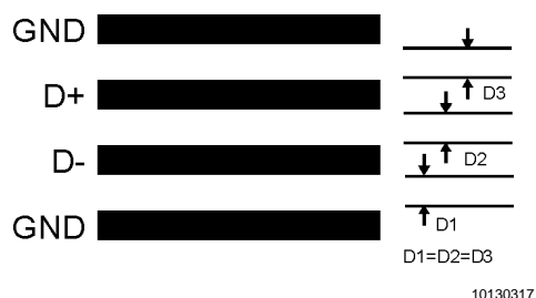
FIGURE 15. Ideal Diode Trace Layout
