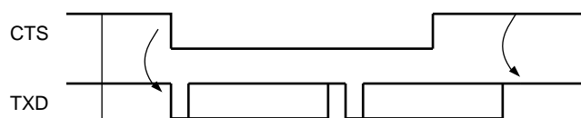
Figure 34-29. Transmitter Behavior when Operating with Hardware Handshaking
