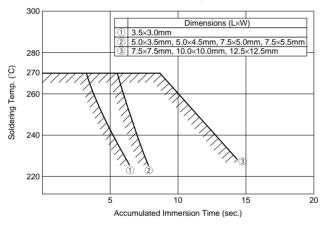
Perform soldering within tolerance range (shaded portion).
