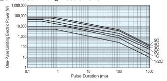
\*The maximum applicable voltage is equal to the max. overload voltage.
