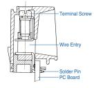
The grooved corners of the pressure plate ensure positive retention of wire(s). The flat bottom of the terminal extends to the inside of the enclosure and connects the terminal to the board(s) inside.
