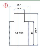
Spring Clamp Solder/Tab Connection
