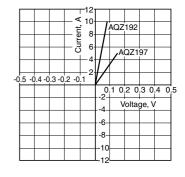
10. Leakage current vs. load voltage characteristics
