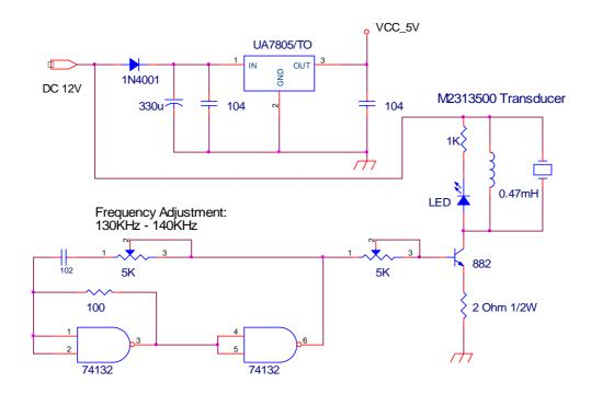
Remark: The negative side faces to the opening, the positive side faces to the liquid source, if driving circuit uses NPN transistor.
