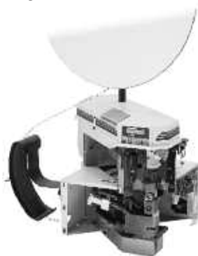
AMP-O-LECTRIC Model "G" Terminating Machine
