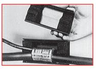
These insulating covers provide hard shell insulated protection for "H" type compression taps and splices and because there is no taping required, you get uniform quality and appearance each time. The exclusive locking design provides the range taking capability. Only five H-tap insulating catalogue cover numbers accommodate the range of 6 AWG – 1000 kcmil in the main and 12 AWG – 500 kcmil in the branch.
