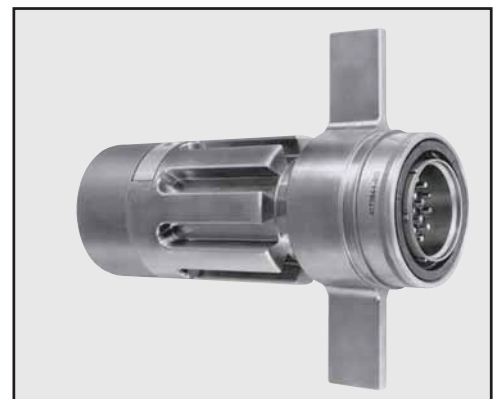
Special configuration Fail Safe used on space telescope application. Lanyard is replaced by a swivel ring for remote disconnect and "wing arms" have been added for manual actuation accessibility by gloved astronauts.
