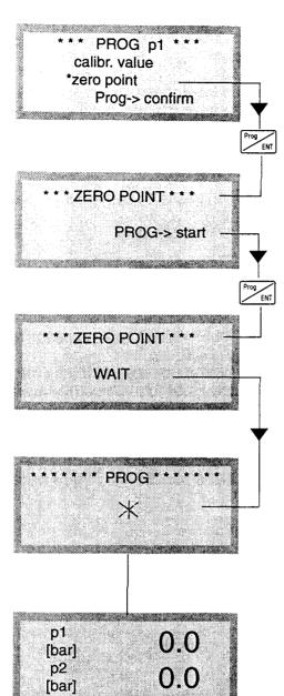
When measuring negative pressures and precise pressure differentials and if the connected pressure sensor has a small zero point deviation, it is advantageous to submit it to a zero point alignment.
