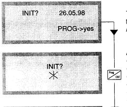
p1 [bar] p2 [bar] The display "INIT" is shown for a short period with a rotating bar. This indicates, that the preadjustments are stored in the EEPROM.
