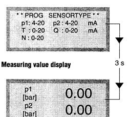
You have the possibility to check which current signals were chosen, when invoking this display with key 0-20. In the example the same current signals were chosen for p1 and p2.
