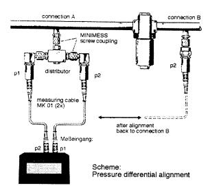
Precise pressure differential measurements are only possible, if an alignment of both pressure sensors was executed first at the same operational pressure level, at which the measurement shall be carried out later.
