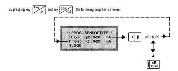
The change-over to 4 to 20 mA is made by a stroke of key  $\left(\begin{array}{c} \Delta \mathbf{p} \\ (p_1 - p_2) \end{array}\right)$ , which is now acting as a cursor and which switches p1 to the
