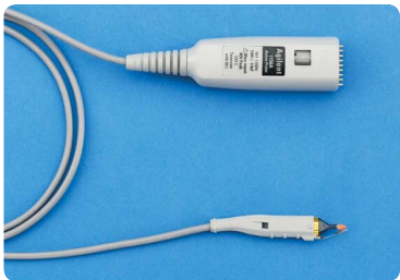
1156A/57A/58A 1.5/2.5/4 GHz active probe
