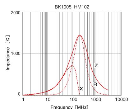
The data is reference only. Electrical characteristics vary depending on environment or measurement condition.
