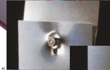
Under equal stress conditions, metal panels bonded with VHB tape show no visible signs of stress compared to those with mechanical fasteners.
