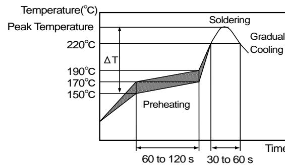
[Allowable Reflow Soldering Temperature and Time]
