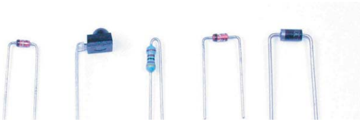
Fig. 3.3 : Parts with bended legs
