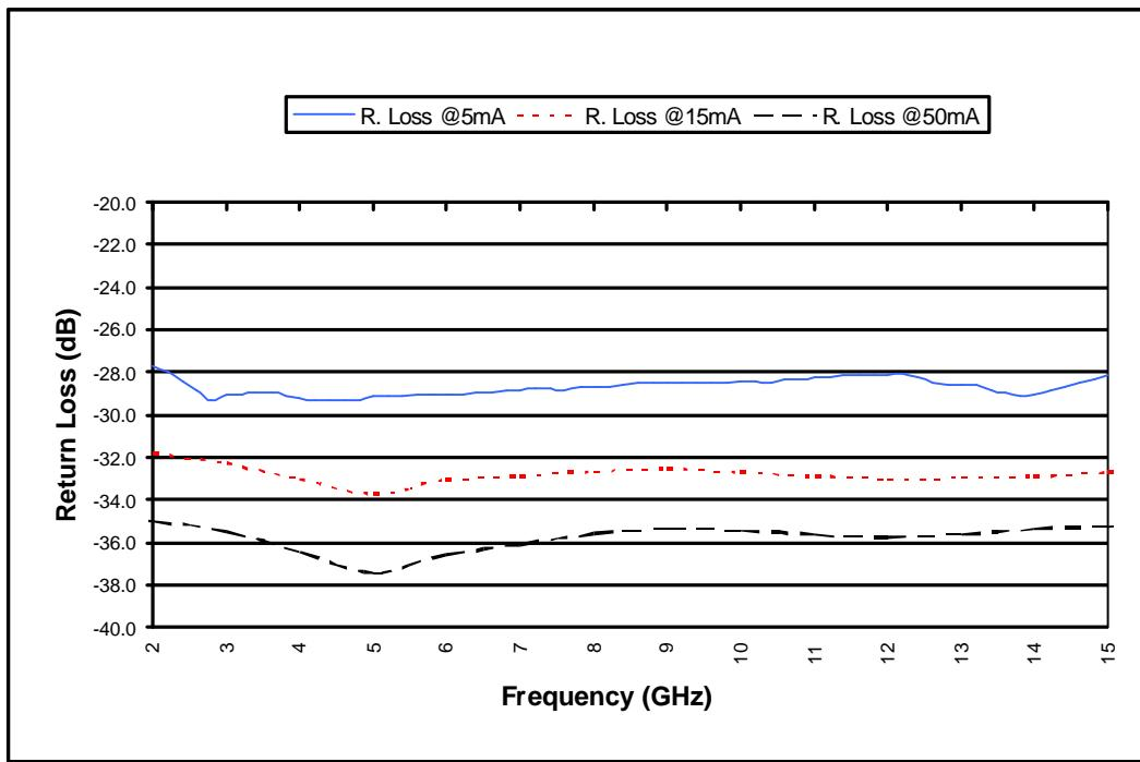
Single Series Diode Isolation vs Frequency
