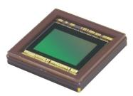
The Toshiba TCM5101ACL is small BSI image sensor.
