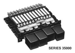
Specify 1 to 18 stations (non-illuminated) with a large selection of mechanical functions, choice of pushbuttons, and up to 6 poles of switching per station. Plungers are on .625" (15.88 mm) centers and are made from .050" (1.27 mm) x .187" (4.75 mm) steel. A square black pushbutton, A592, is supplied with each station. A wide variety of special mechanical functions, features and accessories are also available.
