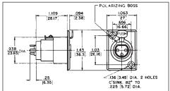
Studio quality black and gold Q-G® receptacle with black housing and gold contacts is designed for low/stable contact resistance and withstands corrosion where highest quality is required for recording and broadcast studio equipment, consoles, and other applications.
