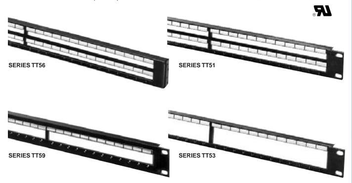
Ten series of blank panels are available in 19" and 23" widths, standard or flush mounting, and double, twin or three row configurations. OEM's can order blank components and individual modules, jacks, switches and lamp jacks for production line assembly according to standard or special front panel configurations. Kwik-Change® designation strips are supplied with panels for custom legend marking. Flush mounting styles can use extension legs (on special
