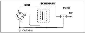
Series 9000 Line Matching Transformers offer low-loss interconnections between high and low impedance equipment. Exclusive mu-metal shielding protects against spurious electrostatic and RF fields. Units are bi-directional and can be used as follows:
