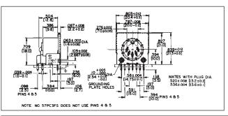
**RIGHT-ANGLE** SHIELDED RECEPTACLE for printed circuit board mounting
