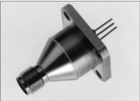
SMA 4 HOLE MOUNTING (REF.: ADA)
