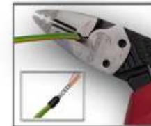
Aderendhülsen crümpen Crimping of ferrules 1,5 - 2,5mm 2
