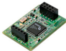
Figure 5: uDiskOnChip Horizontal Version with Dual Connector Configuration
