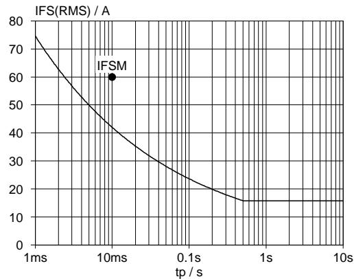
Fig.3. Maximum non-repetitive rms forward current.
