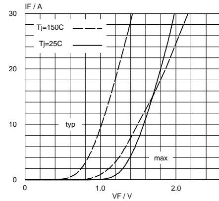
Fig.5. BY359X-1500 forward characteristic  $I_F = f(V_F)$ ; parameter  $T_j$
