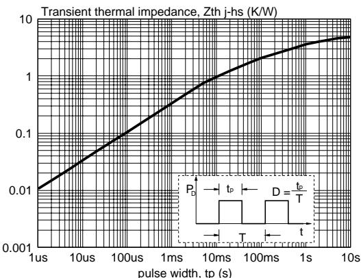
Fig.4. Transient thermal impedance  $Z_{th} = f(t_p)$
