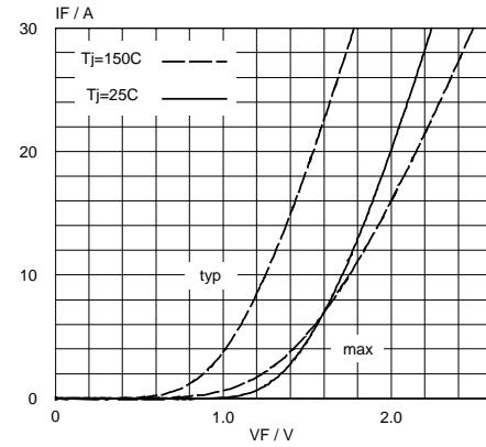
Fig.6. BY359X-1500S forward characteristic  $I_F = f(V_F)$ ; parameter  $T_j$
