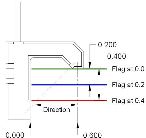
Typical Voltage Output Vs Blocking Distance
