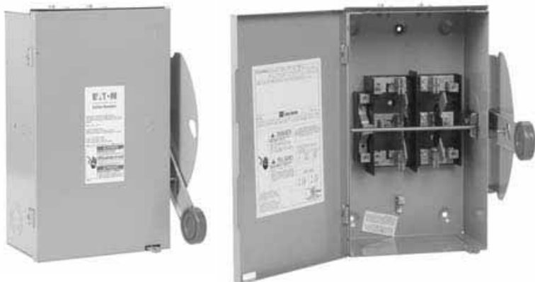
DT223URH-N General-Duty, Non-Fusible Double Throw Emergency Power Safety Switch, 100 Amperes, 120/240 Volts
