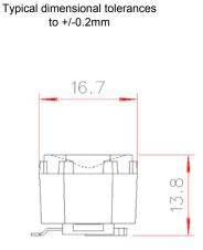
Polymer Optics "Modular LED Optics" design, based on a hexagonal format, allows maximum packing density and assembly flexibility
