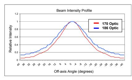
The 186 Diffuse Narrow Angle Collimator can be used with both Standard and Diffuse Moonstone LEDs.
