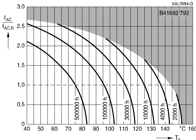
**Useful life<sup>1)</sup>**depending on case temperature  $T_C$  under ripple current operating conditions at  $V_{op}$  $V_R = 25$  V:  $V_{op} \leq 20$  V; $V_R = 40$  V:  $V_{op} \leq 35$  V; $V_R = 63$  V:  $V_{op} \leq 55$  V
