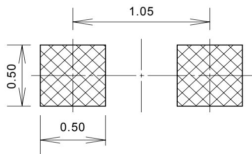
(Note1) Electrode projection is not included in the package dimensions.
